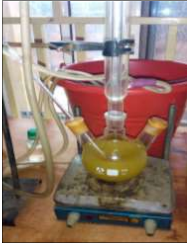
Plate 1: Biodiesel production by transesterification of oil
